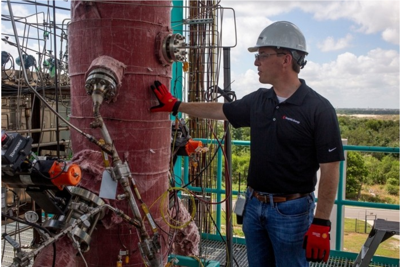
Patrick Hanks, chief technology officer of Graphitic Energy, pats the carbon formation vessel on the company's San Antonio pilot project, which pulls solid carbon graphite out of methane gas. (Dylan Baddour/Inside Climate News)
